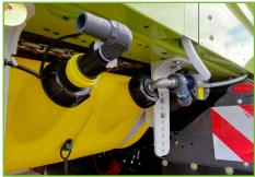
The tank is attached to the body of the wagon. The model of the clamp irons included in the delivery content is universal but the mounting width of the tank can be adjusted by changing the position of the clamps, which means that the tank can be fitted to most wagon models.
