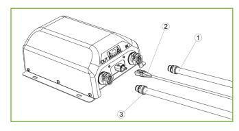
Mount the pump unit firmly with four hex head screws to a suitable place where it is not exposed to unnecessary vibration.
